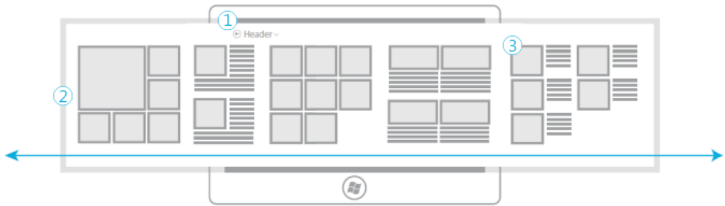
Figure 6-4 The layout of a typical home or hub page of a WinRT app with a fixed header (1), a horizontally pannable section (2), and content sections or categories (3).
